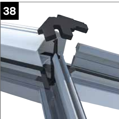
38 ENSURE THE GLASS IS CLEAN AND DRY BEFORE FITTING. Peel back protective film from weathering shield and position (adhesive face down) on glass, locating around the ridge and the hip bars. Press down firmly.
