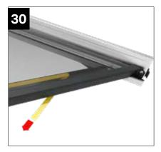
Now the glass is in position and held in place by the glass stops, peel back the remainder of the protective film from the glazing support.
