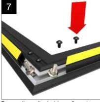
Ensure the mitred rider rail ends are pressed up against each other now fix the cleats into the rider rail using the M5 x 8mm fixings provided through the predrilled holes.
