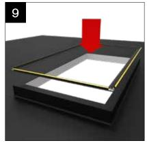
Position the assembled rider rail frame on top of the kerb, centre this rider rail frame over the opening ensuring it is square (check diagonals). Fix down to the kerb using appropriate fixings not supplied.
