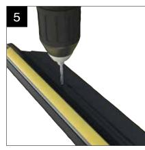
Drill the rider rail at 100mm from each end and drill a minimum of 4 holes at a Max of 400mm centres using appropriate clearance drill. Now take the rider rail and ensure correct number of bolts are slotted into rider rail.
