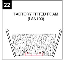
Ensure the foam does not interfere with the clips by pinching it towards the centre of the bar.
