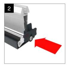
Attach the glazing bar end cap fixing blocks to the transom bars - as access restrictions may prevent easy fixing later. NOTE: These 'snap out' of the end caps when despatched from the factory. These are not required on hip rafters.
