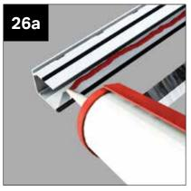
Using MS polymer seal underside of top face of glazing end profile as shown. Depending on the roof specification this can either be a PVCu or Aluminium profile. The end profile is square cut and to be aligned flush with the glazing.
