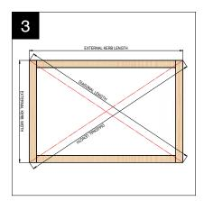
Construct the up-stand to the flat roof with a minimum of 150mm tall kerb (minimum of 70mm wide). Check that kerb is square by measuring diagonals. Ensure the kerb is built to external kerb dimensions that match that specified for the lantern. The customer must ensure that the kerb and surrounding roof can adequately resist
