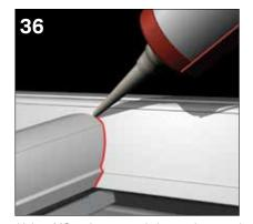
Using MS polymer, seal the gaskets and capping around the joint between the hip bar cappings and the jack rafter cappings.
