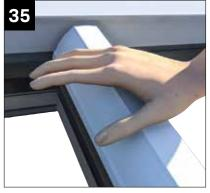
Using the heel of your hand, push down on the top cap to engage the clips, working from ridge to rider rail. Ensure the rubber gaskets are fully compressed for a watertight seal. NOTE: on longer bars it may be necessary to use a soft mallet and timber block.
