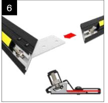
Insert the rider rail cleats into the ends of the mitred rider rail lengths. The cleat should sit inside the PVC sleeve and on top of the aluminium rider rail as highlighted above in red.
