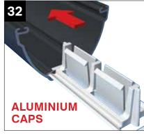
This stage should have been prepped in the factory. If not take the aluminium top caps and lay them onto a protected surface. Slide clips into each bar - position down from ridge at a max centre of 100mm and then at 500mm centres (max) inbetween.
