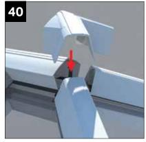
Press firmly down on the ridge end top cap until it clicks into position on the ridge end.
