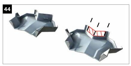
When a central transom between the hips is specified, the internal cover will need the highlighted section above removing. Using a hacksaw cut down the three dotted lines up to the lip. Then using pliers remove the section by bending back and forth. Tidy ends using a small file.
