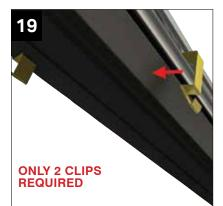
Attach the spring clips (LAN014) to side of the glazing bars. TRANSOM - 2 clips 50mm from the top of the bar. 2 clips 100mm from the rider rail. HIP - 2 clips 100mm from the rider rail.\* top of bar locates on ridge end (see step 21). Push the leg in under the gasket and spring around the underside as shown. Ensure the clips are fully pushed on.
