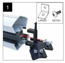
LANRF001 is supplied pre-installed into the bar. Remove and fix radius end (LAN032BL) then replace the screw. If using 3 bar attach LAN031 using EBT001. If aluminium internal claddings are used then these will need to be attached prior to radius end being installed.
