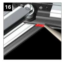
Seal the area where the co-extruded gasket on the hip bar abuts the co-extruded gasket on the jack rafter.
