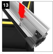
Remove nuts on rider rail. Fit hip bars onto bolts at rider rail end and hand tighten nuts. Ensure the ridge is now level and using an angle finder check the pitch of the lantern is set at 25°.
