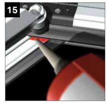
Seal the area where the hip bar abuts the jack rafter as shown above.
