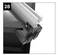
Ensure the glass units are pushed up towards the ridge and that the glazing is securely located behind the glassLOCKs at the hips.
