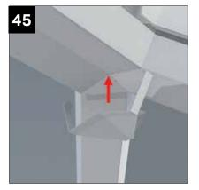
Clip fit into position the aluminium internal radius end cover trim.
